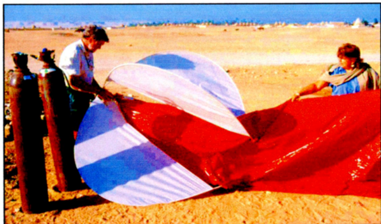
The aerial survey balloon. Filling the replacement balloon envelope for the first time (March 2002). Lift is provided by helium gas.
