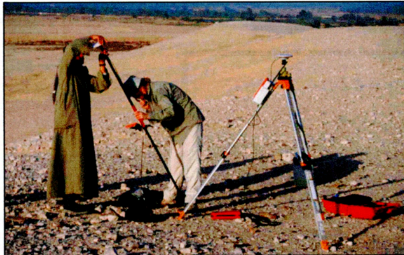
GPS survey of the Amarna hinterland (March 2002). Surveyor Helen Fenwick sets up the differential GPS equipment above the Workmen's Village.
