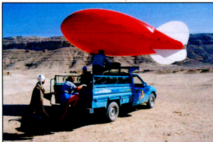
The aerial survey balloon. For taking it greater distances it can be towed by a small truck.
